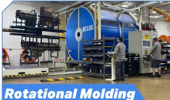
Complex shapes that allow for our tank designs are best achieved with in-house equipment. We own multiple dual station rotational molding machines that allow us to produce finished parts from raw plastic. Producing consistently higher quality parts, and respond quickly to sales spikes.
