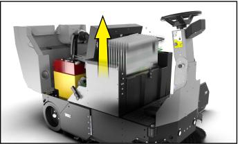
Remove screws and metal strips
